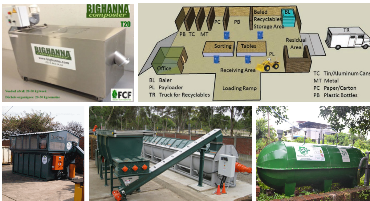
Figure 7: Examples of containerised composting (left-up, left-down and middle down), small scale material recovery and transfer station (right-up) 3 and small-scale bio-digester (right-down) 4
